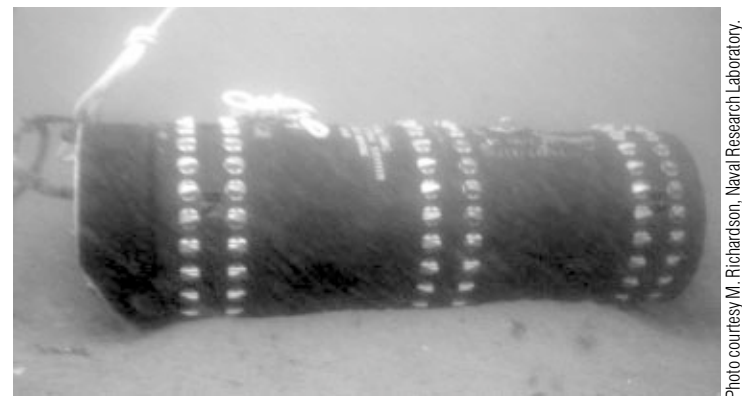
Researchers use inert instrumented mines to study mine burial.
