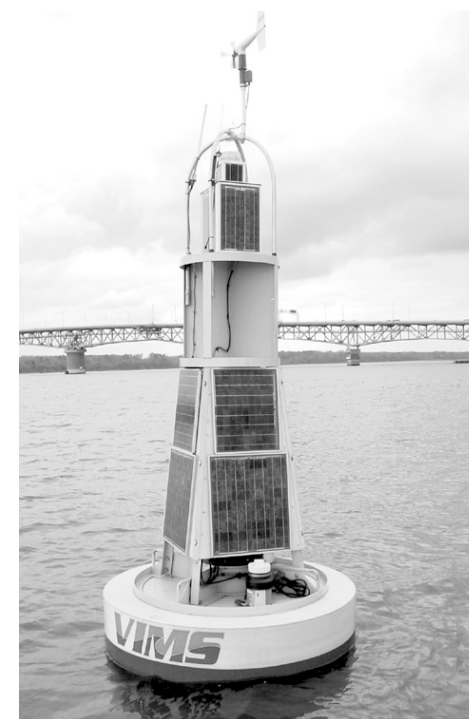
Solar panels power the sensors aboard VIMS’ new research buoy.
