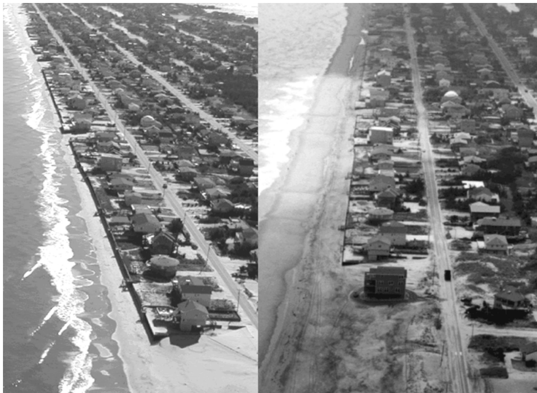
Sandbridge, Virginia (just south of Virginia Beach) before (L) and after (R) beach nourishment. The beach is much wider in the after-nourishment photo, even though that photo was taken after Hurricane Isabel.
