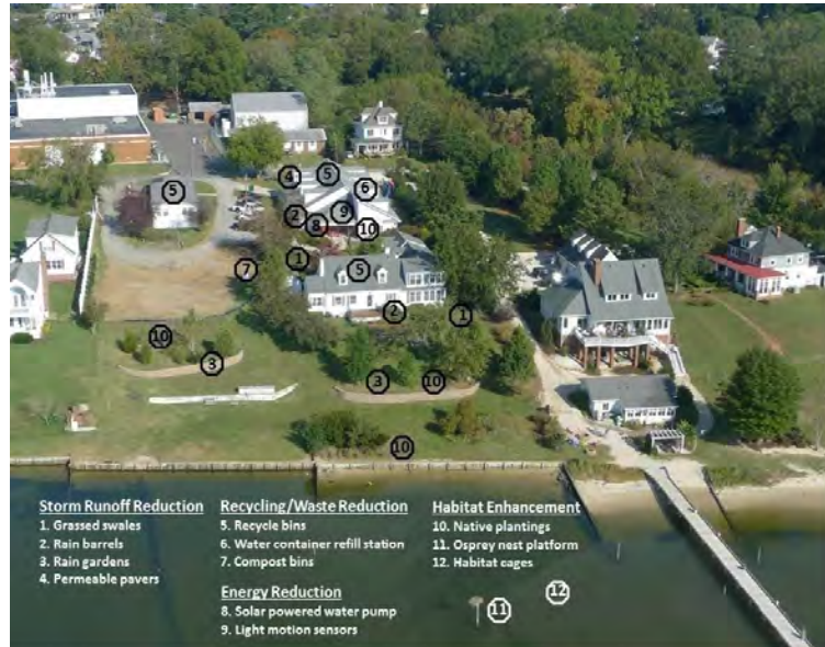
Figure 11.2. Aerial view of CBNERR-VA facilities and infrastructure at VIMS Gloucester Point campus highlighting design elements promoting good environmental stewardship, with a specific focus on residential options. Image source: VIMS.
