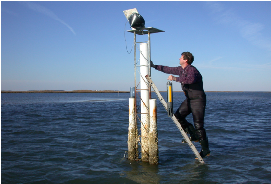
Servicing a SWMP Station (photo credit: NOAA / NERRS photo library)
