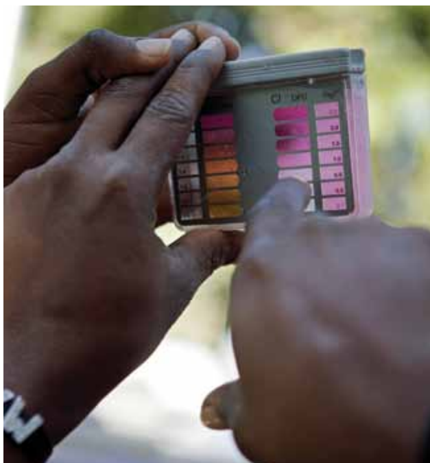
Testing the chlorination level in the water distributed in a camp next to the neighborhood of Cite de Dieu in Port-au-Prince.
