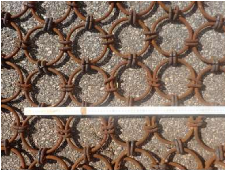
Figure 1. Rings fastened together with 2 split links per side.
