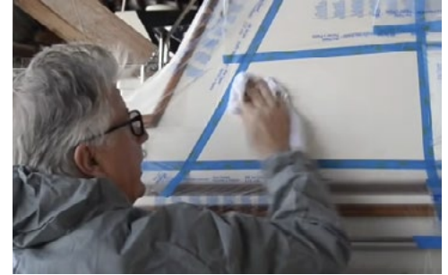
BoatUS shows you how to use a disposable sprayer to repair gelcoat.
