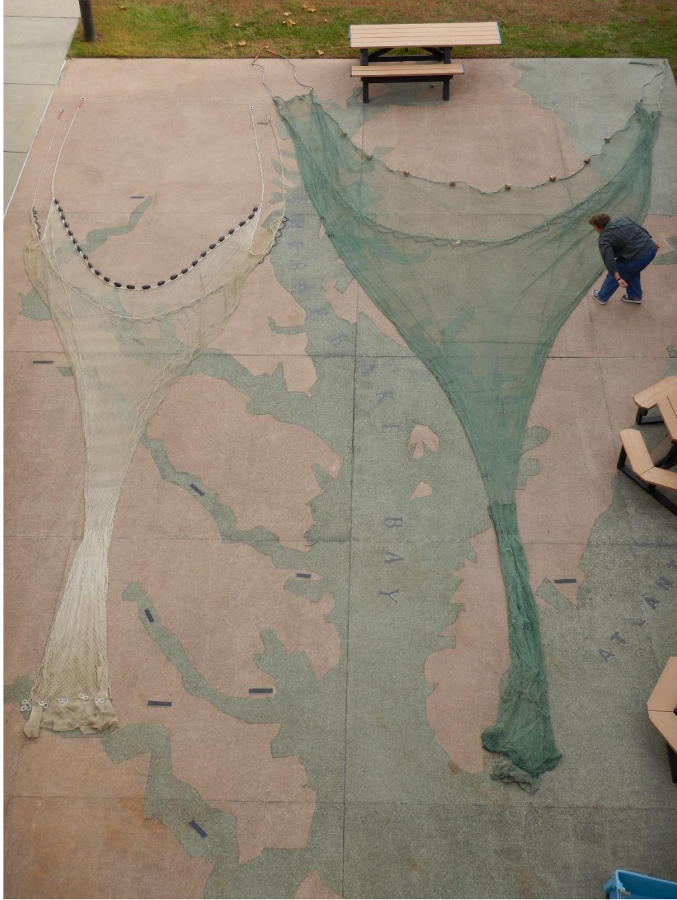
Figure 1. The new trawl with a 5.8-m head line, 40 mm stretch-mesh body, and a 6.4-mm liner used aboard the R/V Tidewater (Left), and the 9.1-m head line, 4-seam, semi-balloon otter trawl with 38.1 mm stretch-mesh body and a 6.4-mm mesh cod liner used to collect fishes from the R/V Fish Hawk (Right).
